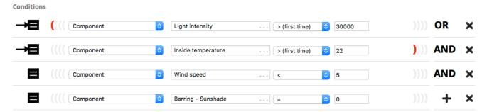
In this second example, the action is initiated when either the light intensity or the inside temperature rises above the set values, but only when the wind speed is below 5 (m/s) and the barring option is not active.
