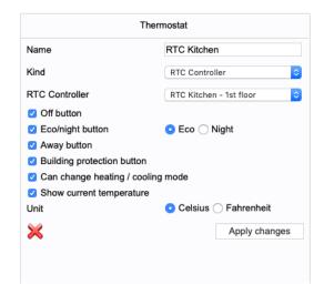
For every RTC element, you can select which options you want to allow in the visualization. These options, together with the parameters of the RTC you have set up, will define the possibilities you have in the xxter app.
